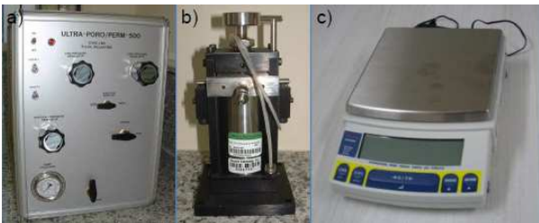
Figure 3 - Equipments used for grain density and porosity measurements: a) gas poropermeameter; b) matrix cup; c) semi-analytic precision scale.
