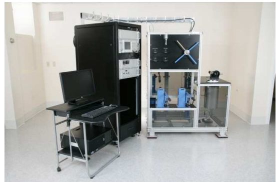
Figure 4 - System used for measuring of rock elastic properties.
