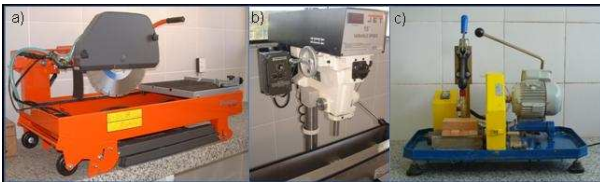
Figure 2 - Equipments used for plug preparation: a) saw; b) portable diamond bit engine drill; c) plug rectifier.
